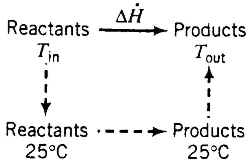
(a) Process path for heat of reaction method
