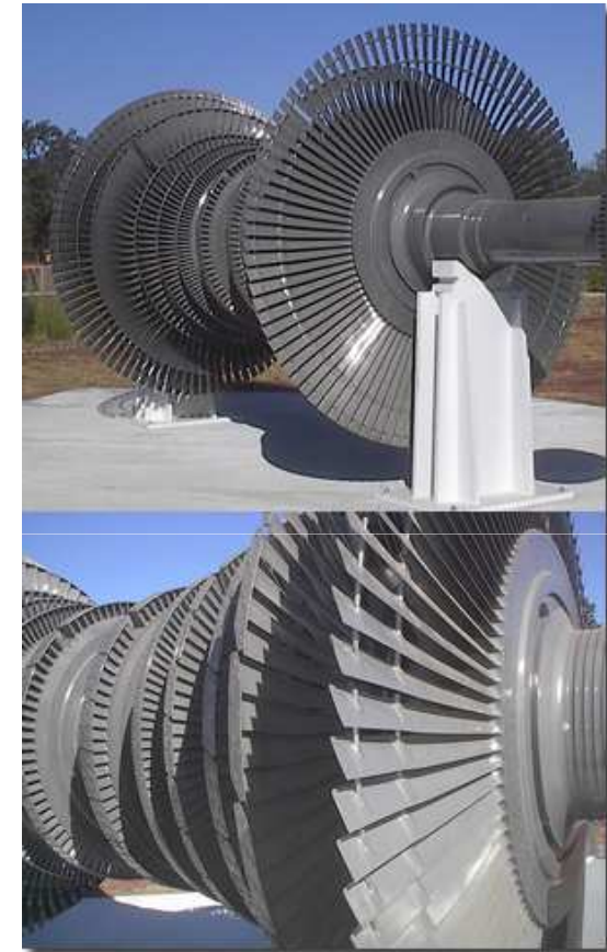
Steam Turbine Blades from a Calpine Geothermal Plant DKB
