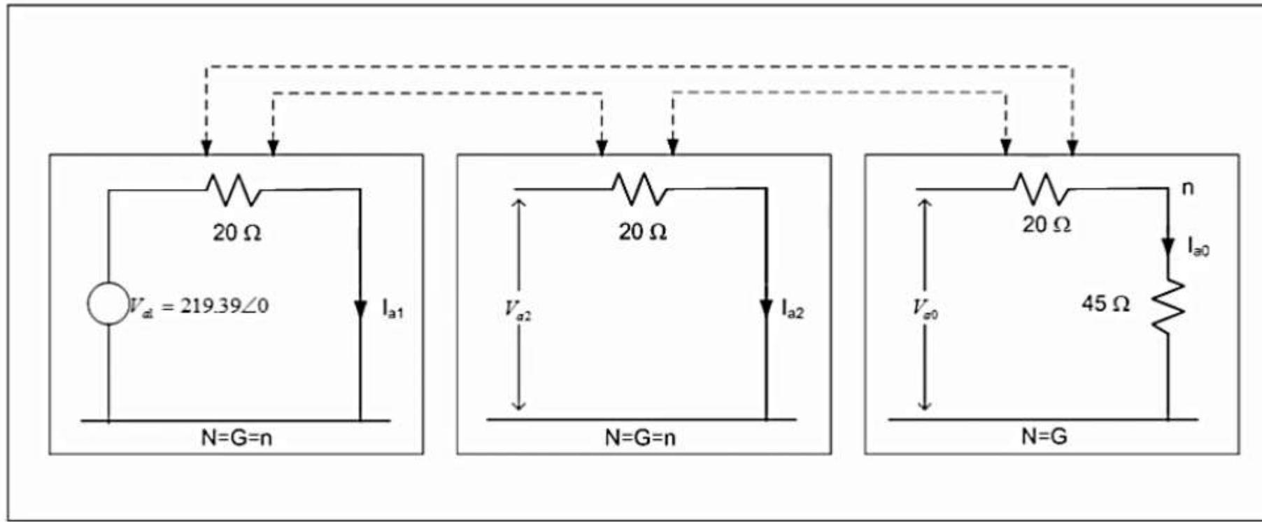
$$\begin{bmatrix} V_{a1} \\ V_{a2} \\ V_{a0} \end{bmatrix} = \begin{bmatrix} 219,3931\angle 0 \\ 0 \\ 0 \end{bmatrix} \quad Z_{120 \text{ (total)}} = \begin{bmatrix} 20 & -5 + j2,8868 & -5 - j2,8868 \\ -5 - j2,8868 & 20 & -5 + j2,8868 \\ -5 + j2,8868 & -5 - j2,8868 & 65 \end{bmatrix}$$
