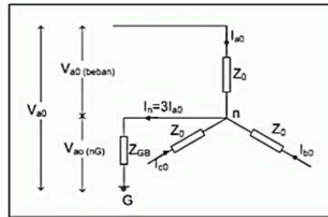
$$I_{a0} = \frac{1}{3}(I_a + I_b + I_c) \quad I_{a0} = \frac{1}{3}I_n \quad I_n = 3I_{a0}$$
