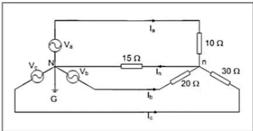
$$[V_{abc}] = \begin{bmatrix} V_a \\ V_b \\ V_c \end{bmatrix} = \begin{bmatrix} 219.3931\angle 0 \\ 219.3931\angle -120 \\ 219.3931\angle 120 \end{bmatrix} \quad [V_{120}] = [A^{-1}] [V_{abc}]$$
