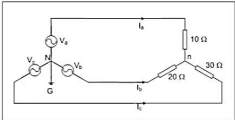
$$\begin{aligned}[V_{120}] &= \begin{bmatrix} V_{a1} \\ V_{a2} \\ V_{a0} \end{bmatrix} = \begin{bmatrix} 219.3931\angle 0 \\ 0 \\ 0 \end{bmatrix} \\ Z_{120(\text{total})} &= \begin{bmatrix} 20 & -5 + j2,8868 & -5 - j2,8868 \\ -5 - j2,8868 & 20 & -5 + j2,8868 \\ -5 + j2,8868 & -5 - j2,8868 & \infty \end{bmatrix} \end{aligned}$$
