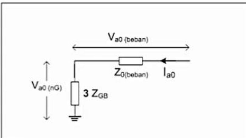
$$V_{nG} = V_{a0(nG)} = Z_{GB}I_n = 3Z_{GB}I_{a0}$$
