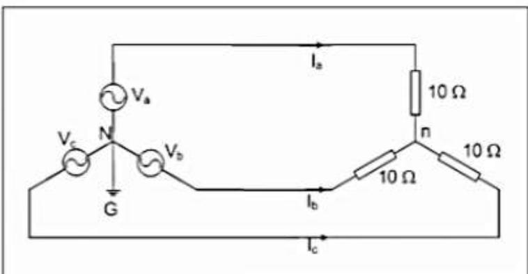
$$\begin{aligned}V_a &= 180\angle 0 \\V_b &= 250\angle -90 \\V_c &= 220\angle 100\end{aligned}$$
