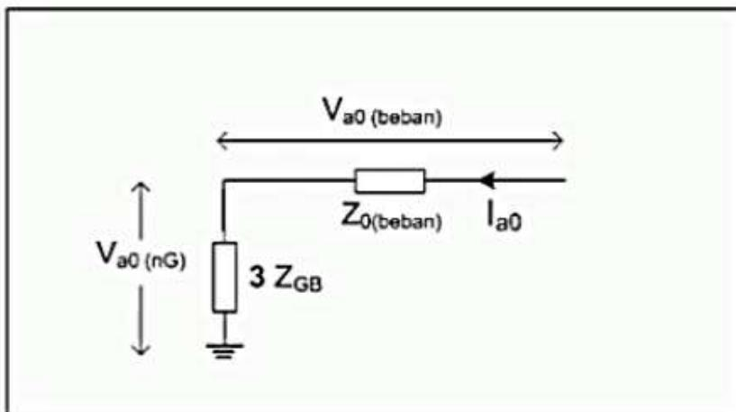
$$V_{nG} = V_{a0(nG)} = Z_{GB}I_n = 3Z_{GB}I_{a0}$$
