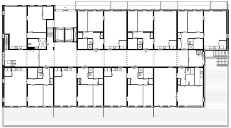
Figure 23. Extra wide corridors and small windows looking out into them were designed to 'stimulate' socializing among residents. (Source: HVDN Architects)
