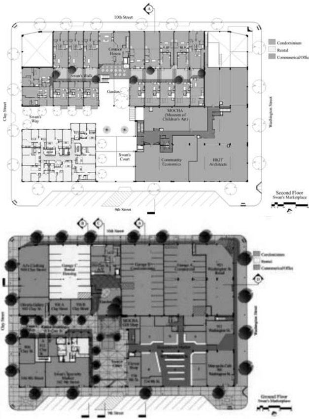
Figure 3. Swan's Market, site plan. The cohousing entrance and common garden are located on the ground floor, off Swan's court. The condominium entrances are located on the second floor. (Source: Pyatok Architects)
