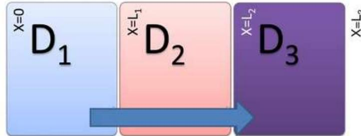
$$\frac{\partial C}{\partial t} = D \frac{\partial^2 C}{\partial x^2}$$
