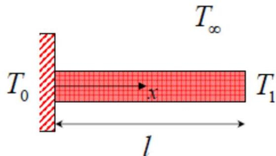
$$\frac{d^2T}{dx^2} - \frac{hP}{kA}(T - T_\infty) = 0$$
