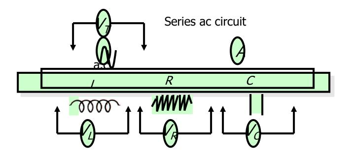
Consider an inductor *L*, a capacitor *C*, and a resistor *R* all connected in series with an ac source. The instantaneous current and voltages can be measured with meters.
