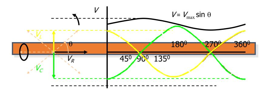
Rotating phasor diagram generates voltage waves for each element R, L, and C showing phase relations. Current i is always in phase with  $V_R$
