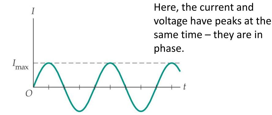
In order to visualize the phase relationships between the current and voltage in ac circuits, we define phasors – vectors whose length is the maximum voltage or current, and which rotate around an origin with the angular speed of the oscillating current.
