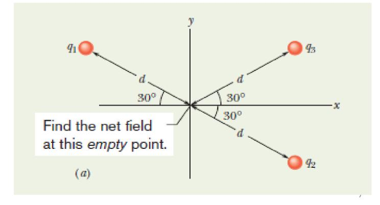
Charges q1, q2, and q3 produce electric field vectors E1, E2, and E3 respectively, at the origin, and the net electric field is the vector sum E = E1 + E2 + E3. To find this sum, we first must find the magnitudes and orientations of the three field vectors.
