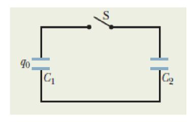
$$q_0 = C_1 V_0 = (3.55 \times 10^{-6} \,\text{F}) (6.30 \,\text{V})$$
