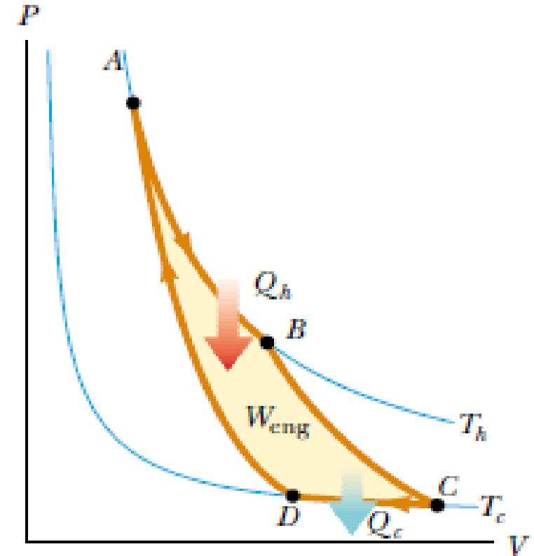
1. Process  $A \rightarrow B$  is an isothermal expansion at temperature  $Th$ . The gas is placed in thermal contact with an energy reservoir at temperature  $Th$ . During the expansion, the gas absorbs energy  $|Qh|$  from the reservoir through the base of the cylinder and does work  $WAB$  in raising the piston.
