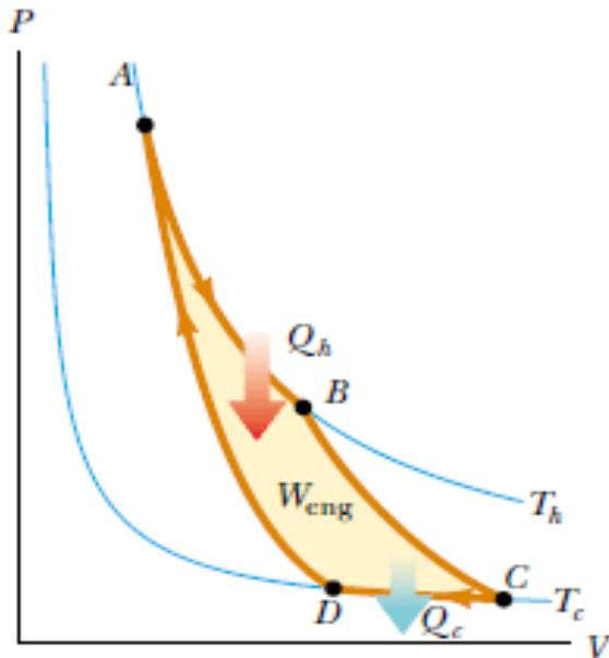
3. In process  $C \rightarrow D$ , the gas is placed in thermal contact with an energy reservoir at temperature  $T_c$  and is compressed isothermally at temperature  $T_c$ . During this time, the gas expels energy  $|Q_c|$  to the reservoir, and the work done by the piston on the gas is  $W_{CD}$ .
