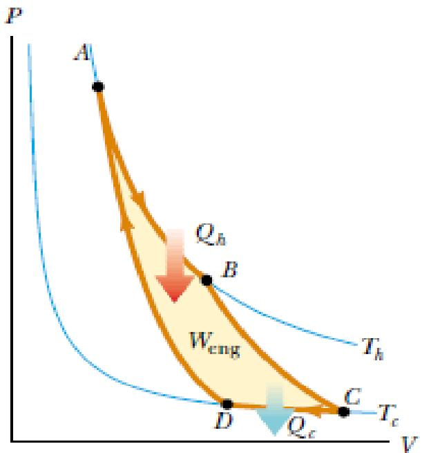
2. In process  $B \rightarrow C$  the base of the cylinder is replaced by a thermally nonconducting wall, and the gas expands adiabatically—that is, no energy enters or leaves the system by heat. During the expansion, the temperature of the gas decreases from  $T_h$  to  $T_c$  and the gas does work  $W_{BC}$  in raising the piston.
