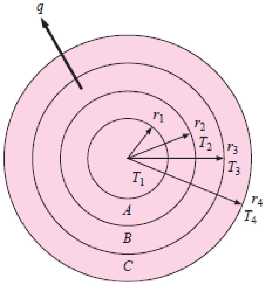
$$\frac{q}{R_A} = \frac{\ln(r_2/r_1)}{2\pi k_A L}$$
