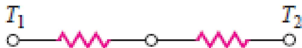
$$\frac{\ln(r_2/r_1)}{2\pi k_s L} \quad \frac{\ln(r_3/r_2)}{2\pi k_a L}$$
