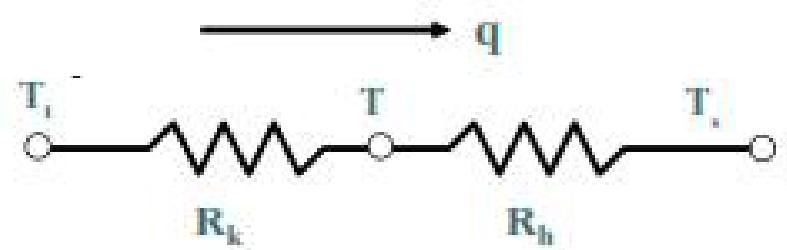
$$R_k = \frac{\ln(r_c/r_i)}{2\pi k L} \quad R_h = \frac{1}{2\pi r_c L h}$$
