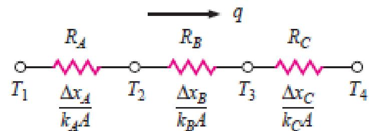
$$q = \frac{T_1 - T_4}{\Delta x_A/k_A A + \Delta x_B/k_B A + \Delta x_C/k_C A}$$
