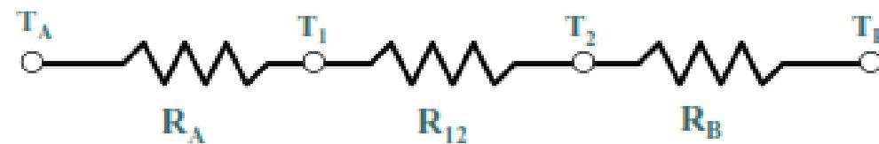
$$q = \frac{T_A - T_B}{\frac{1}{h_1 A} + \frac{\Delta x}{kA} + \frac{1}{h_2 A}} = \frac{A(T_A - T_B)}{\frac{1}{h_1} + \frac{\Delta x}{k} + \frac{1}{h_2}}$$
