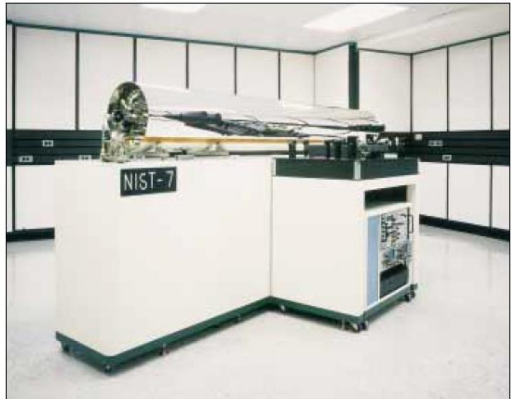
Figure 1.1 (Top) The National Standard Kilogram No. 20, an accurate copy of the International Standard Kilogram kept at Sèvres, France, is housed under a double bell jar in a vault at the National Institute of Standards and Technology (NIST). (Bottom) The primary frequency standard (an atomic clock) at the NIST. This device keeps time with an accuracy of about 3 millionths of a second per year. (Courtesy of National Institute of Standards and Technology, U.S. Department of Commerce)
