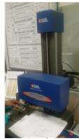
Dilakukan pengujian roughness di Quality Assurance PT.SK Indonesia
