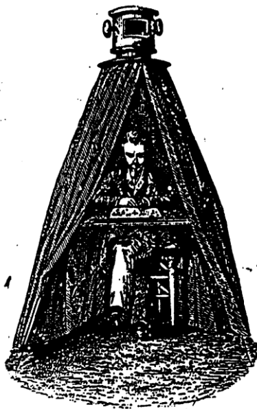
3 Nineteenth-century tent camera obscura, of the type used by Johannes Kepler in 1620.
