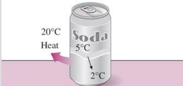
(b) An impossible heat transfer process
