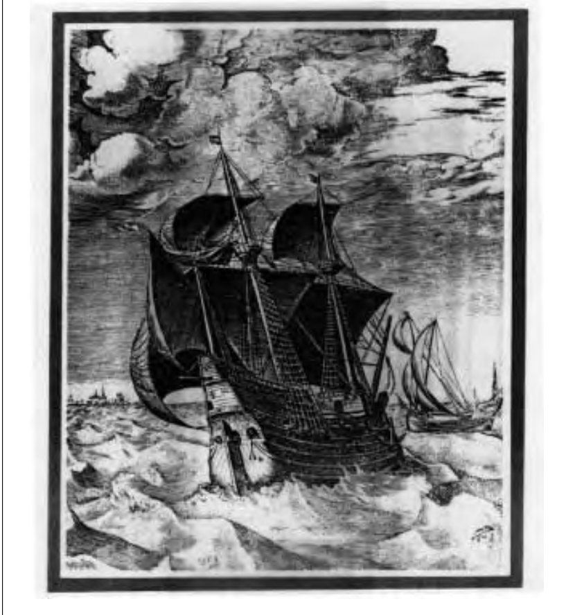
Figure 7-1. “A Flemish version of the machine with which the {European mariners } changed the world: the three-masted ship, square-rigged on the foremast and main-mast, lateen-rigged on the mizzemast, with smaller vessel in sight” (Crosby, 1986: Plate 2).
