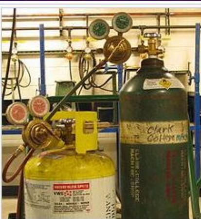
Industrial compressed gas cylinders used for oxy-fuel welding and cutting of steel.
