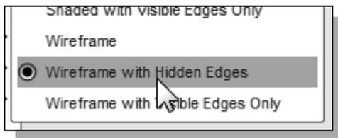
The *Wireframe Image* display option allows the display of the 3D objects using the basic wireframe representation scheme.
