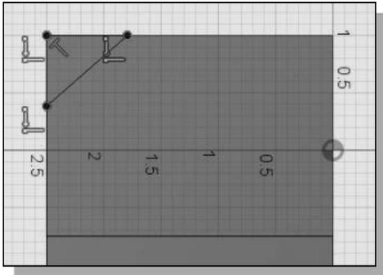
4. Start at the upper left corner and create **three line segments** to form a small triangle as shown.
