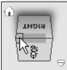
9. Move the cursor over one of the corners of the **ViewCube** and drag with the left-mouse-button to activate the **Free Rotation** option.
