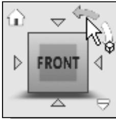
3. Move the cursor over the counter-clockwise arrow of the **ViewCube** and notice the orbit option becomes highlighted.
