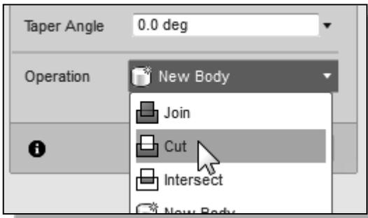
11. Select the **CUT** option in the *feature option* list to set the extrusion operation to *Cut*.
