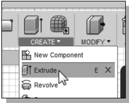
1. In the *Create toolbar*, select the **Extrude** command by clicking the left-mouse-button on the icon as shown.
