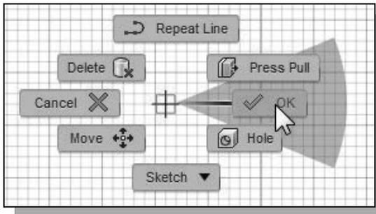
2. Inside the graphics window, click once with the **right-mouse-button** to display the option menu. Select [**OK**] in the pop-up menu, or hit the [**Esc**] key once to end the Sketch Line command.
