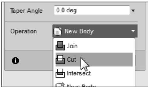
10. Select the **CUT** option in the *feature option* list to set the extrusion operation to *Cut*.
