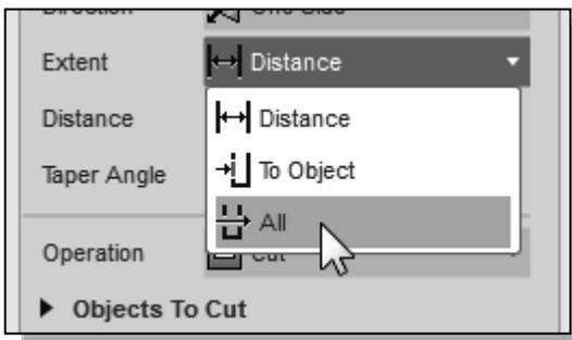
14. Set the *Extent* option to **Through All** as shown. The *All* option instructs the software to calculate the extrusion distance and assures the created feature will always cut through the full length of the model.
