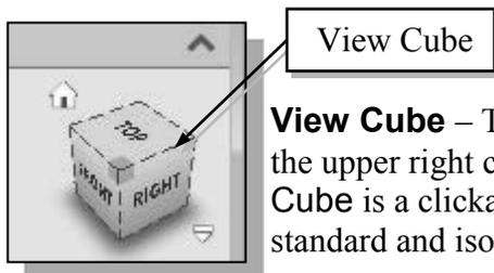
**View Cube** – The View Cube is a 3D navigation tool that appears at the upper right corner of the *Fusion 360* main window. The View Cube is a clickable interface which allows you to switch between standard and isometric views.
