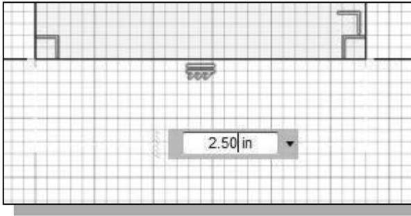
2. In the *Edit Dimension* window, the current length of the line is displayed. Enter **2.5** to set the length of the line.
