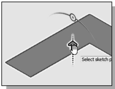
12. Move the cursor on top of the arrow; notice the dashed line appears as shown. We can drag the arrow, with the left mouse button, to set the extrusion distance and direction.
