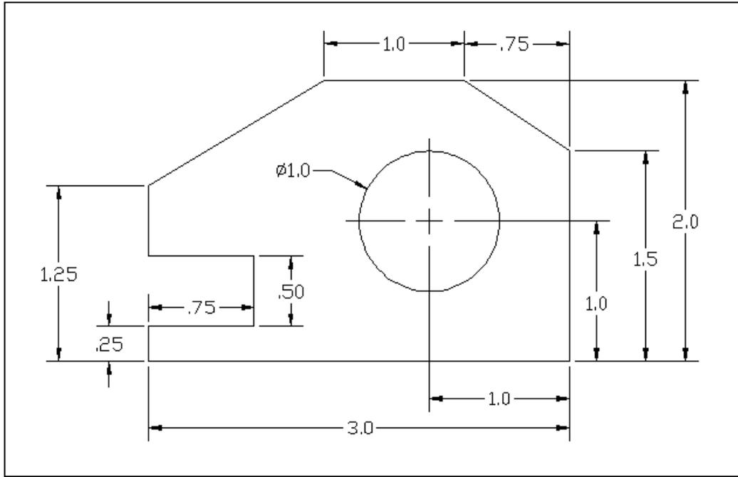
2. **Spacer Plate (Thickness: .125)**
