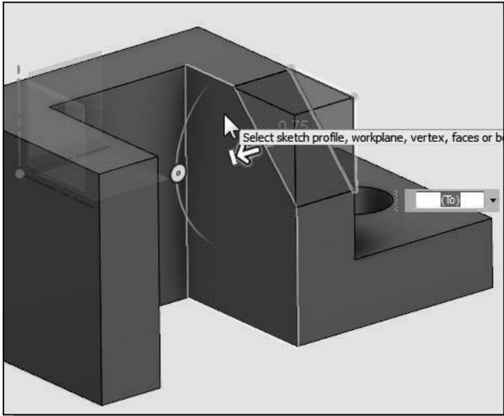
12. On your own, use the dynamic rotate function and select the back surface as shown.
