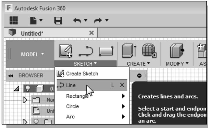
1. Move the graphics cursor to the **Line** icon in the *Sketch* toolbar. A *Help-tip box* appears next to the cursor and a brief description of the command is displayed at the bottom of the drawing screen: “*Creates lines and arcs.*”
