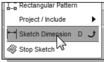
6. Select the **Sketch Dimension** command in the *Sketch* toolbar. The Sketch Dimension command allows us to quickly create and modify dimensions. You can also hit [D] on the keyboard to activate this command.
