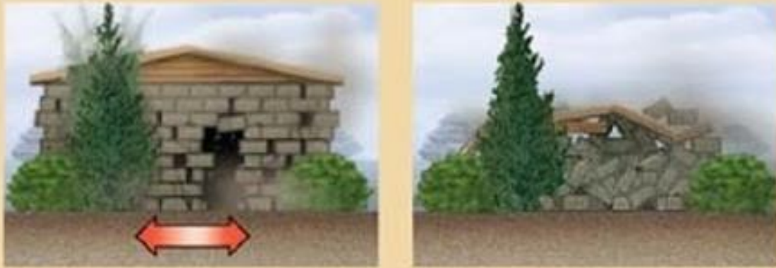
(d) A neighborhood of masonry buildings in Armenia collapsed during a 1999 earthquake because the walls broke apart.
